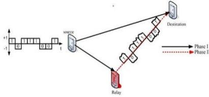
Figure 4 Amplify and forward relay
